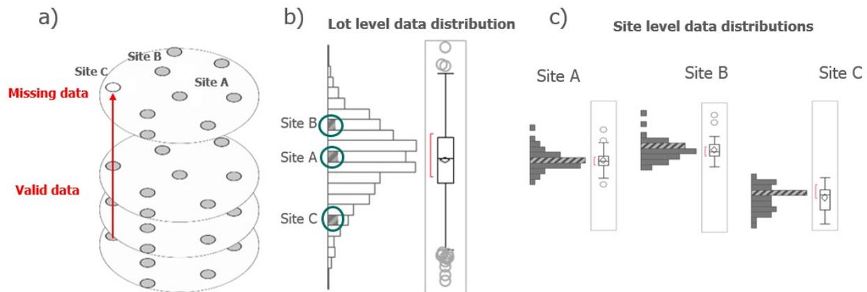
Figure 10 (a) schematic representation of site level data aggregation within large wafer set. (b) distribution of total data set with markups on the site level (c) the site level data distribution referenced in sketch (a) and histogram (b).
