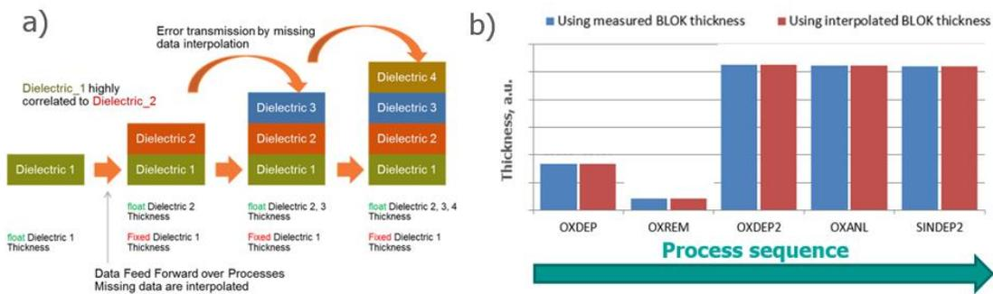
Figure 6 (a) Schematic representing missing data input and error propagation; (b) Comparison of the real vs virtual data input based on the nearest-neighbor interpolation scheme.
