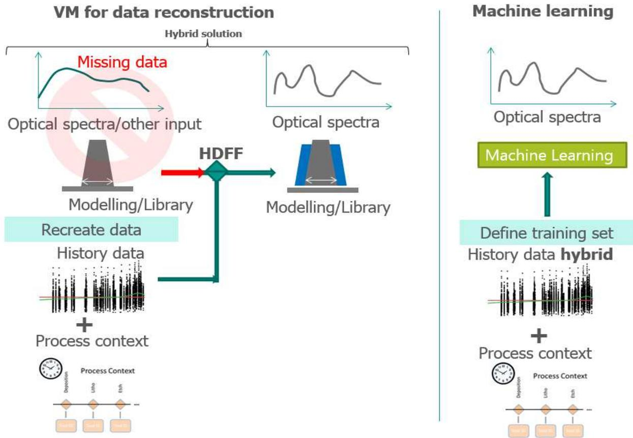
Figure 8 Concept of two approaches to solve the problem of missing HDFS data: virtual metrology and machine learning
