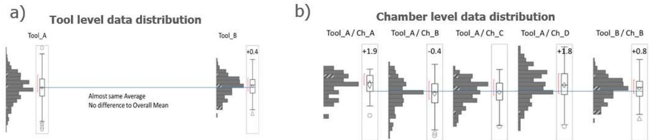
Figure 11 Statistical distribution for the same data set for two data aggregation levels: a) tool level, b) chamber level.
