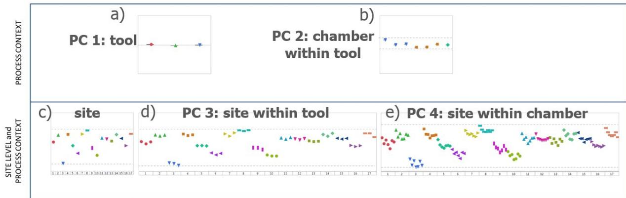
Figure 12 Data reconstruction using context-based virtual metrology: a) the etch-tool level, b) the etch-chamber level, c) the site level (no process context), d) the site level data on the tool level, and e) the site level data for the etch-chamber level.
