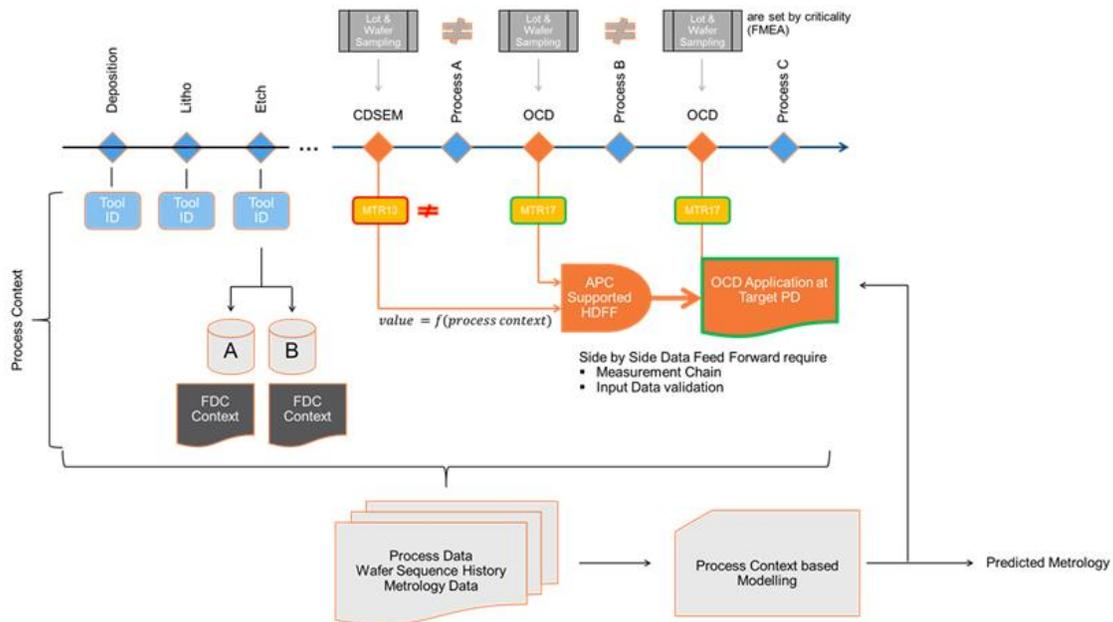
Figure 3 Schematic representation of information flow utilizing virtual metrology.
