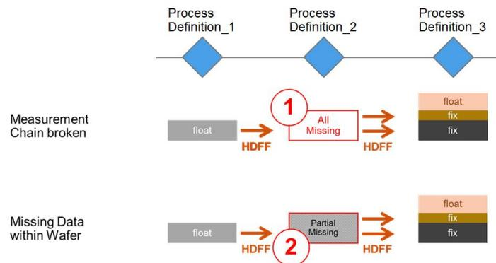
Figure 1 Examples of hybrid data feed-forward (HDFF) approach. Top picture shows HDFF scenario with incomplete data due to missing whole-wafer data. The picture at the bottom displays situation where the measurements of particular sites within the wafer are missed.
