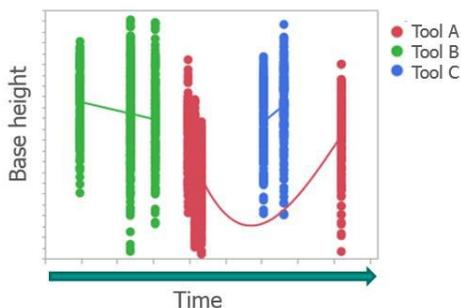
Figure 14 Tool data within studied set vs data acquisition time. Product-level data shows also different performance. The data reconstruction should be done on the product level.
