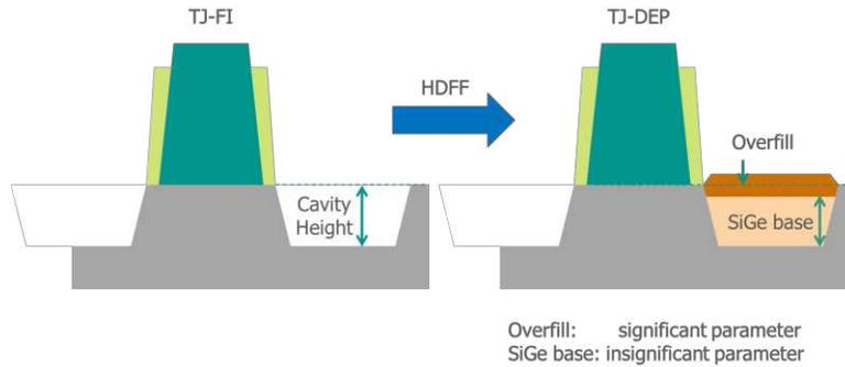
Figure 9. Schematic representation HDFF configuration. Cavity depth and other dimensions as TJ-FI are passed to TJ-DEP step.
