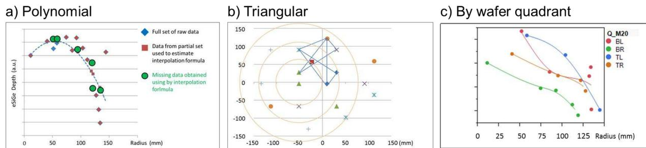
**Figure 5.** (a) Radial distribution interpolated by second-order polynomial function; (b) Triangular interpolation approach for missing data, and (c) comparison of triangular interpolation data per wafer quadrant vs wafer radius. The symbols in panels b) and c) denote respective wafer quadrants: TL (top left), TR (top right), BL (bottom left), and BR (bottom right).
