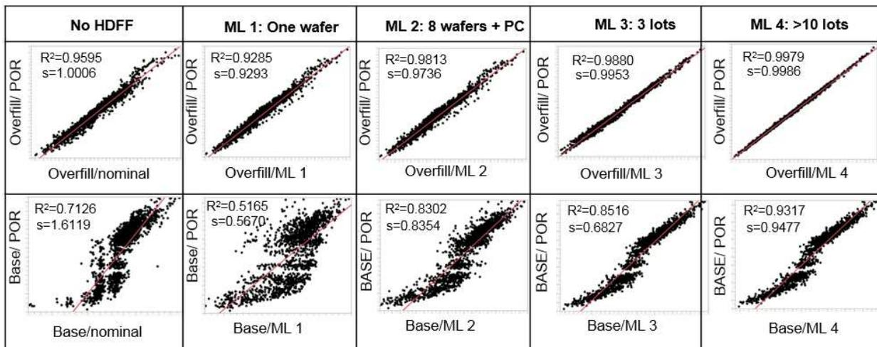
Figure 15 Correlation of POR hybrid production data for overfill and base parameters of TJ-DEP HDFF application: (No HDFF) the hybrid data were missing and interpretation was done with nominal values; (ML4) with training set larger than 10 lots; (ML 2) training with three wafer lots; (ML 3) training with eight wafers chosen based on process context knowledge, and, finally, (ML 1) training with single wafer.
