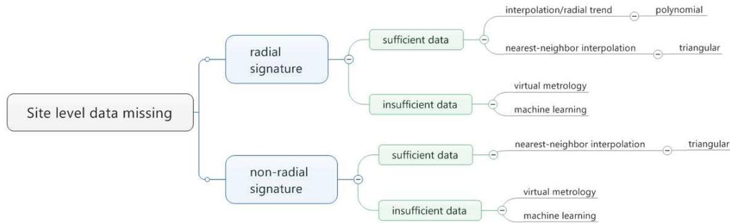
**Figure 4** Schematic representation of missing data recreation scheme when site level data is missing
