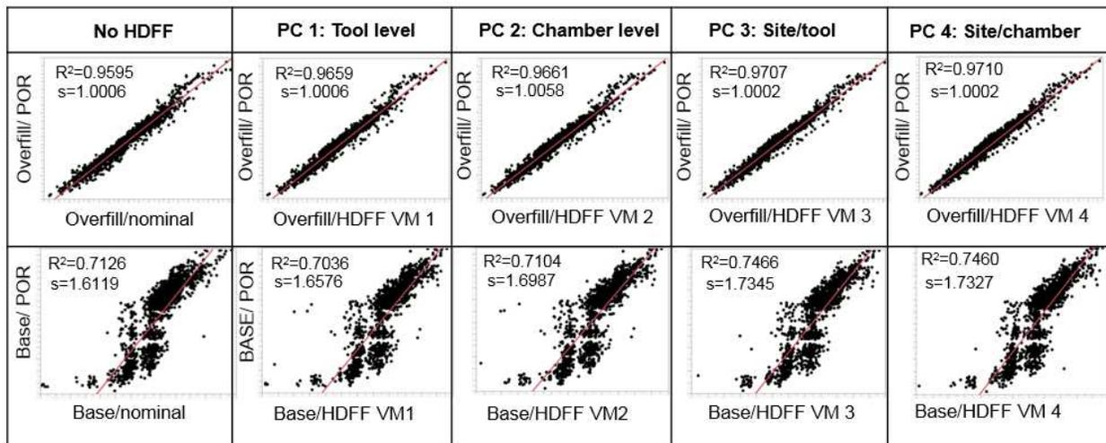
Figure 13 Correlation of the POR hybrid production data for overfill and base parameters of TJ-DEP application: (No HDFS) the hybrid data were missing and interpretation was done with nominal values; (PC1) the data were reconstructed on the tool level; (PC2) the data were reconstructed on the chamber level, (PC3) the data were reconstructed on both site and tool levels, and, finally, (PC4) the data were reconstructed on the site/chamber level.
