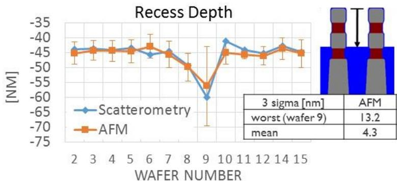
**Figure 8. OCD shows a good agreement with the AFM results at the wafer center. AFM measured a limited sampling of only 6 trenches. The AFM 3 sigma error bar indicates the trench variability. The OCD averages a few hundred trenches within the collection spot and therefore does not have a corresponding error bar. The OCD precision is well below 1nm for the recess depth parameter.**
