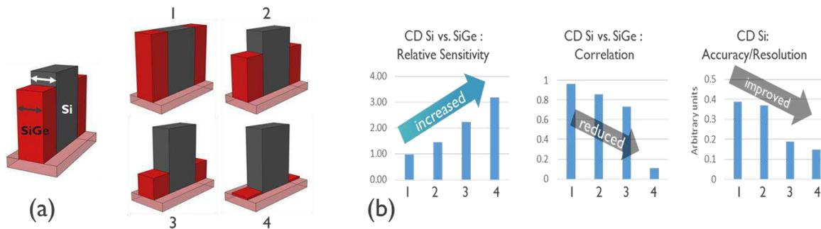
**Figure 11. (a) The toy model and its four configurations. (b) Toy model theoretical analysis, showing improvement of Silicon metrology performance as the SiGe box size decreases relative to the Silicon box.**
