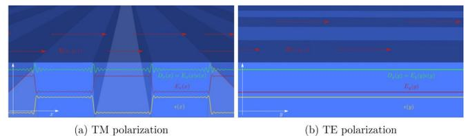
Fig. 5. TM (-s) and TE (-p) polarization at a one-dimensional grating (modulation along x): a) TM (-s) polarization causes unphysical oscillations at the grating slopes resulting in bad convergence behavior b) TE polarization without jump discontinuities. The schematic is shown only for illustrative purpose (the wave propagation is more complex in the studied application).
