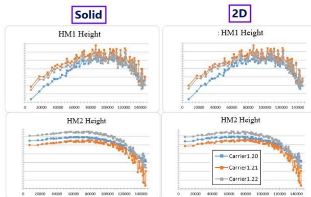
Fig. 7. HM1 and HM2 height radial plots obtained using RCWA model interpretation. Data for solid measurement pad (left hand side) and two-dimensional structure (right hand side).
