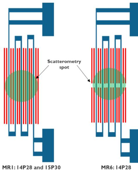
Figure14. Schematic of different meanders and the scatterometry spot size.
