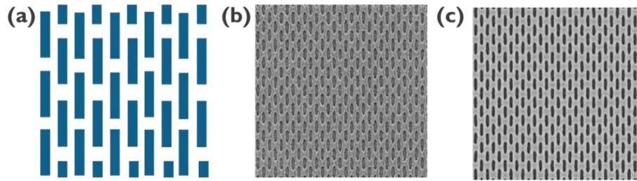
Figure 7. Schematic of the staggered block arrays (a) ADI printed pattern (b), AEI pattern etched into HM (c)
