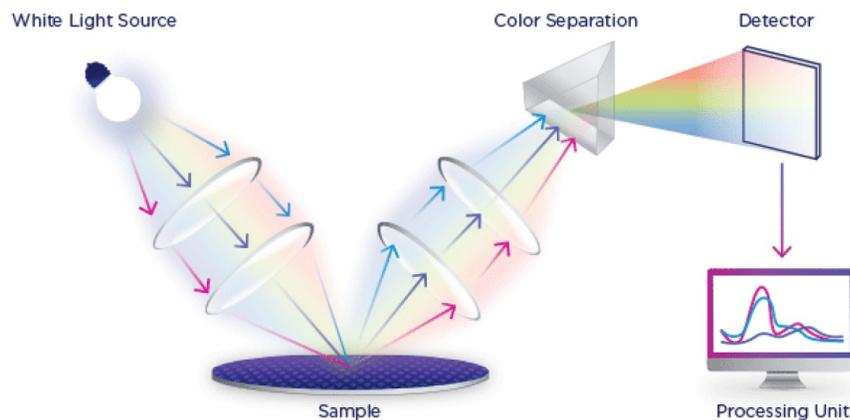
Figure 1 Schematic of scatterometry spectra collection and data analysis
