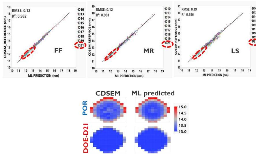
Figure 6. (Top) AEI Correlation plots between CDSEM reference versus ML prediction. (Bottom) AEI wafer maps for two CDU wafers (different etch conditions)
