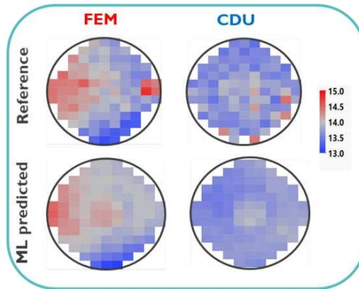
Figure 4. ADI wafer maps for FEM and CDU wafers: top CDSEM reference, bottom - ML solution.
