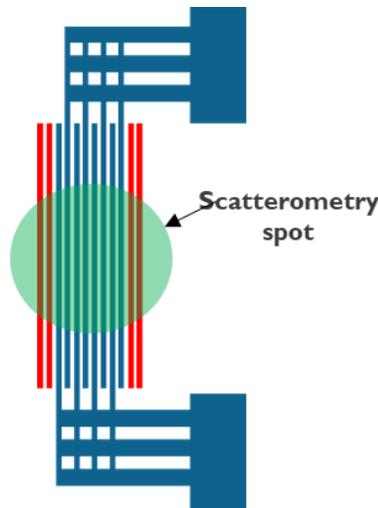
Figure12. Schematic of the FF size and the scatterometry spot size.
