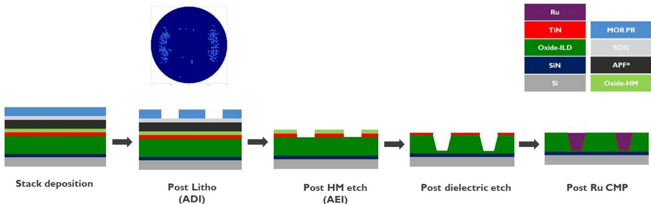
Figure 2 Process flow, stack and source map
