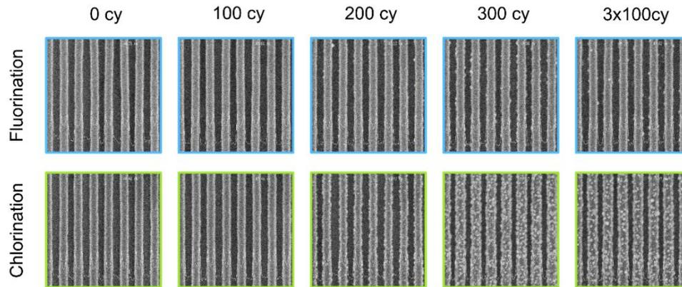
Figure 3. Top-down SEM images of 90 nm pitch a-C:H line pattern after plasma halogenation and deposition of ALD TiO<sub>2</sub> within a single process (100 cycles, 200 cycles, 300 cycles) or via three ALD supercycles (3x100 cycles).
