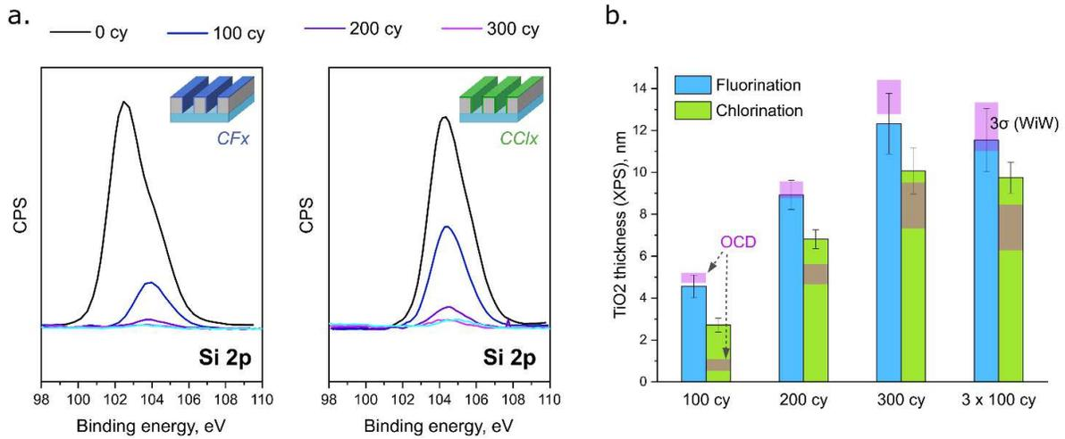
Figure 6. XPS analysis of the ASD TiO<sub>2</sub> process on the growth area (SiN<sub>x</sub>) in the 90 nm pitch a-C:H line pattern: (a) evolution of Si 2p peak induced by deposition of ALD TiO<sub>2</sub>; (b) TiO<sub>2</sub> thickness estimated via attenuation of Si 2p peak intensity and corresponding OCD TiO<sub>2</sub> thickness.
