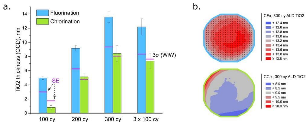
Figure 4. OCD analysis of the ASD TiO<sub>2</sub> process on the growth area (SiN<sub>x</sub>) at the 90 nm pitch a-C:H line pattern: (a) OCD TiO<sub>2</sub> thickness in comparison with the results of spectroscopic ellipsometry (SE) measurements performed at SiN<sub>x</sub> pattern-free areas of the same wafer; (b) OCD TiO<sub>2</sub> thickness wafer map.
