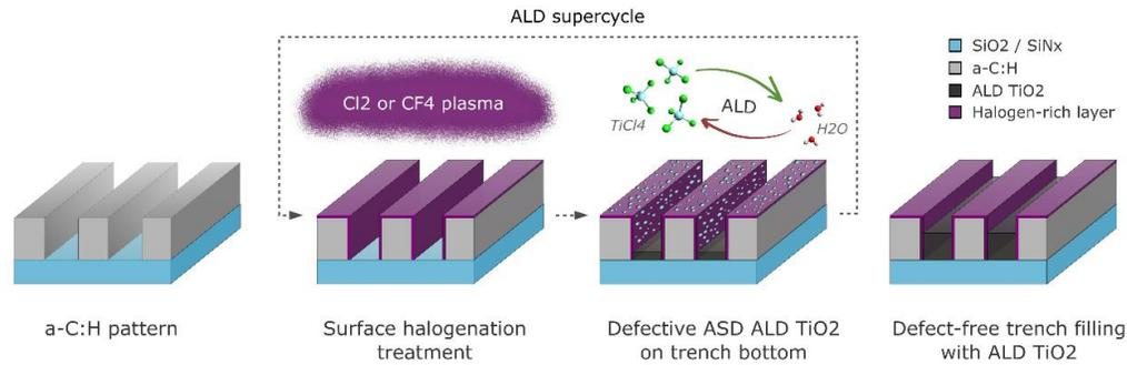
Figure 1. The proposed approach for area-selective deposition of ALD TiO<sub>2</sub> featuring plasma halogenated amorphous carbon as a non-growth surface and an ALD supercycle scheme based on intermediate halogenation plasma treatment.
