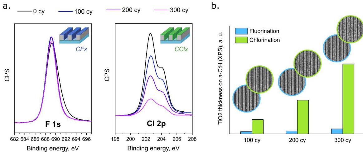
Figure 7. XPS analysis of the ASD TiO<sub>2</sub> process on the non-growth area (halogenated a-C:H) in the 90 nm pitch a-C:H line pattern: (a) changes in F 1s and Cl 2p signals induced by deposition of ALD TiO<sub>2</sub> on the surface of fluorinated and chlorinated a-C:H lines, respectively; (b) TiO<sub>2</sub> thickness estimated via attenuation of F 1s and Cl 2p signals.
