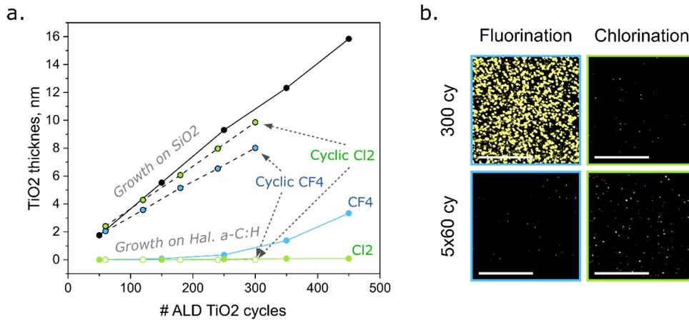
Figure 2. Selectivity and defectivity of the proposed ASD ALD TiO<sub>2</sub> process tested on blanket films: (a) thickness of ALD TiO<sub>2</sub> measured on SiO<sub>2</sub> and on halogenated amorphous carbon surfaces with RBS; (b) defect map obtained from AFM topography images by threshold marking (5σ), the scalebar on the images is 500 nm.
