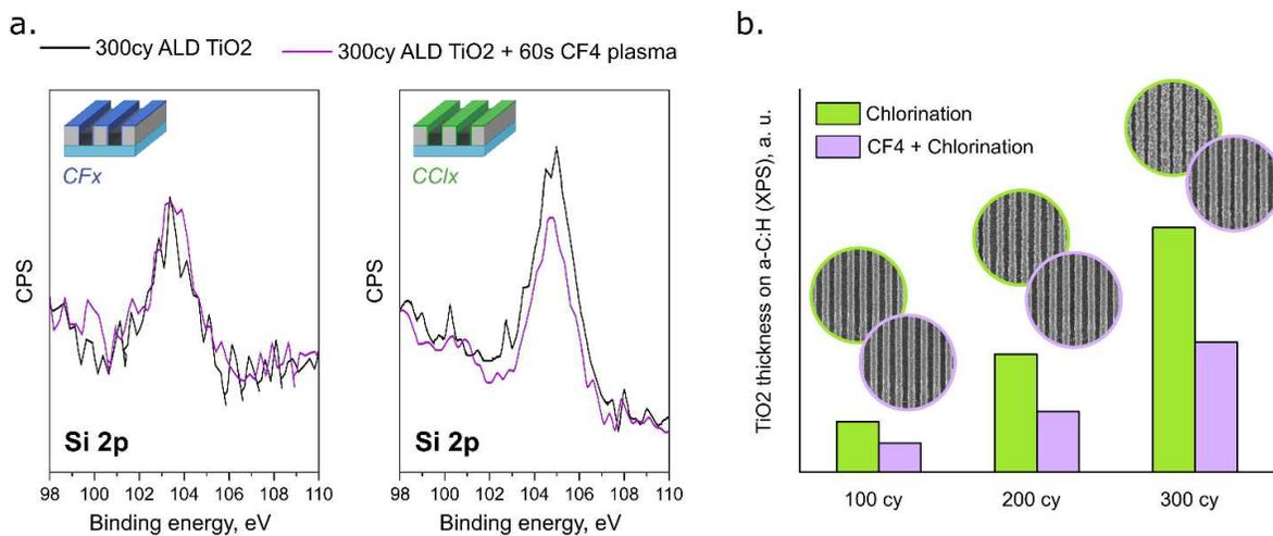
Figure 8. Adverse effect of hard-mask residues on selectivity of ALD TiO<sub>2</sub> process featuring chlorinated a-C:H line pattern: (a) Si 2p XPS signals recorded after deposition of 300 cycles ALD TiO<sub>2</sub> and after additional exposure to CF<sub>4</sub> plasma; (b) the effect of CF<sub>4</sub> plasma pre-treatment on the TiO<sub>2</sub> defects formed over the non-growth area (chlorinated a-C:H) assessed by XPS and top-down SEM.
